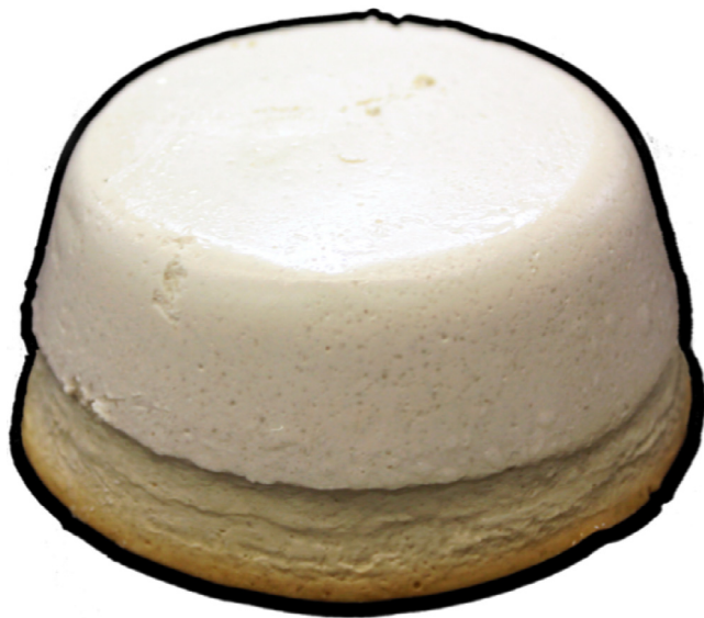
Fig. 3. Synthetic bait comprised of chemo-attractant formulation in calcium-sulfate soluble matrix.
